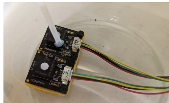
Abb. 5: Elektrochemische H_2S -Sensoren in geschlossener Glaskammer Fig. 5: Electrochemical H_2S sensors in closed glass chamber
